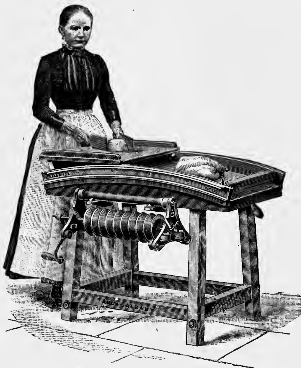
Fig. 65.—“Arch-Albany” Butter Worker, showing the Making-up Board in position, and the Roller when not in use.
